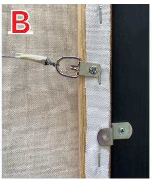
**D-Rings** are best for attaching wire to the back of the frame (screw eyes stick out and damage the walls).
